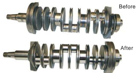
All Outboard crankshafts and wrist pins that we polish are measured, inspected and cleaned before polishing. Once polished they get a coat of rust preventative prior to shipment. Shown above is, before polishing and after.
