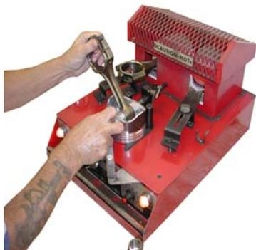
**Press Wrist Pins On and Off Rods**
