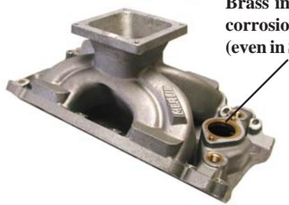
Brass inserts for corrosion resistance (even in Salt Water)
