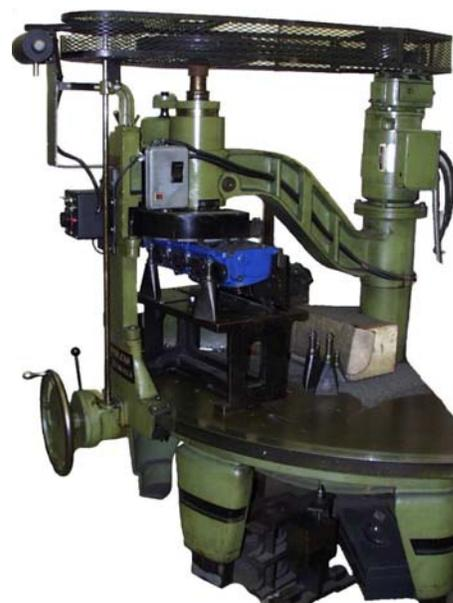
**Inboard Block & Cylinder Head Decking**
