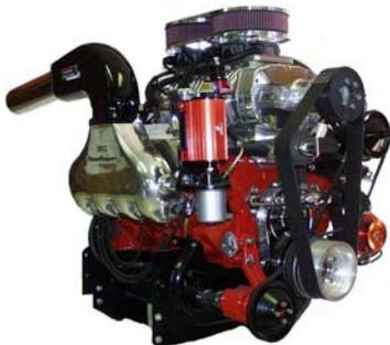
The Blower Shop low profile 250 polished super charger kit with twin GM TBI fuel injection, Delco electronics, Spark control, and fuel system. Shown on an 8.9L 540 CID 700+ HP Flagship GM marine engine
