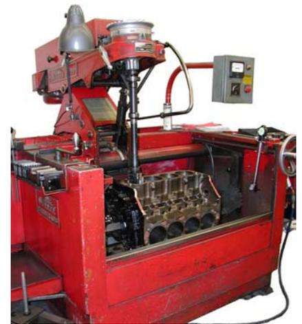
**Inboard Engine Block Honing**
