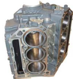
**Suzuki 4 Cycle Cylinder Boring**
